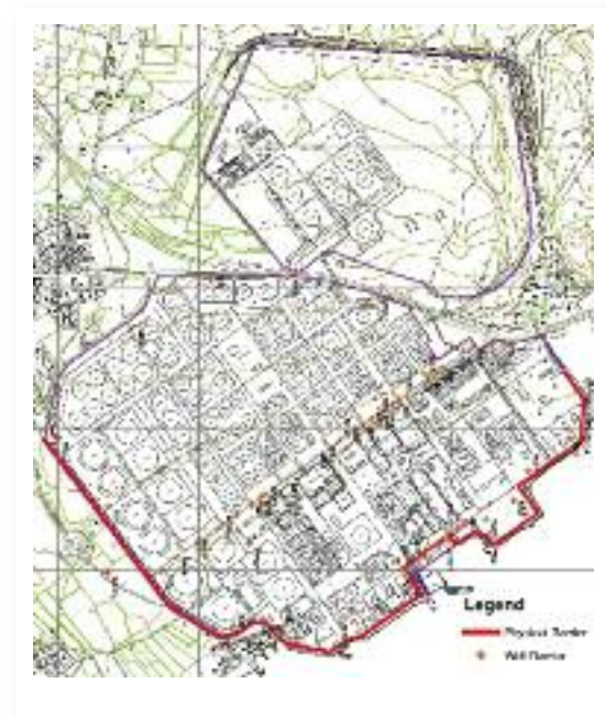
Figure 6 – Location of physical and dynamic barrier under construction
