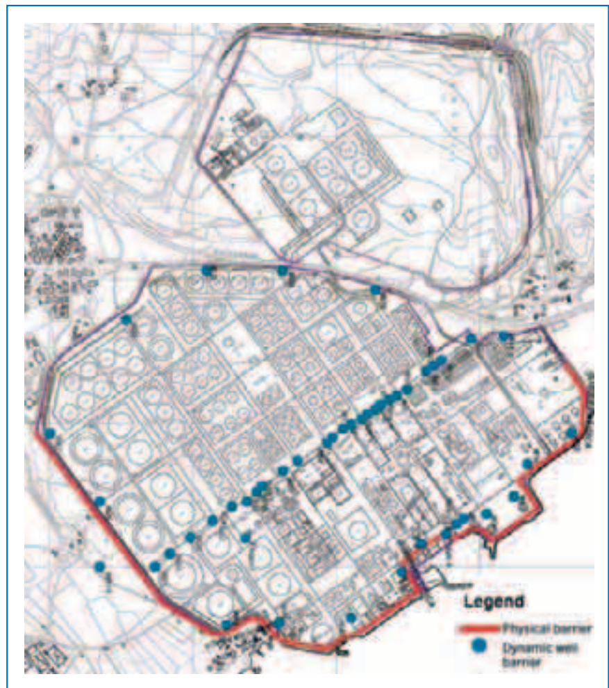
FIGURE 19 Location of the wells comprising the dynamic barrier, and planned location of the physical barrier
