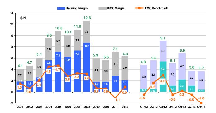
Refining Margin: (comparable EBITDA Refining + Fixed Costs) / Refinery runs in the period IGCC Margin: (EBITDA IGCC plant + Fixed Costs) / Refinery runs in the period EMC Benchmark: margin calculated by EMC (Energy Market Consultants) with 50% Urals – 50% Brent crude oil slate
