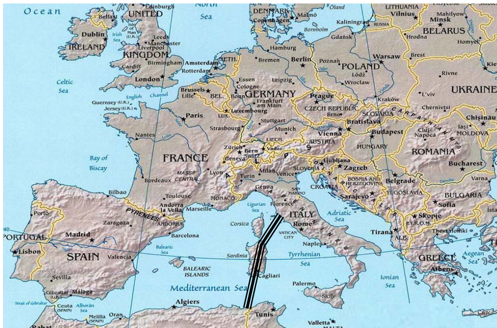
=== GALSI Pipeline: new infrastructure connecting Algeria (near Skikda) with Italy (Piombino) through Sardinia, total capacity of 8 Bcm/y with start-up in 2015
